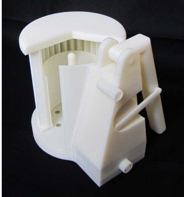
Figure 3. A multiple-barrier hand-held water treatment device that provides protection against a range of microorganisms including viruses, bacteria, and protozoa. Hand power conveys the water through the device and provides electricity to operate a UV disinfection system.
