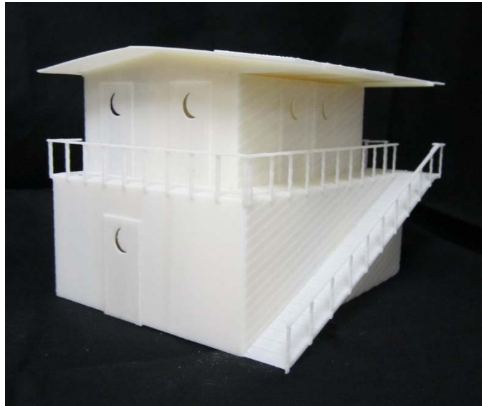
Figure 5: This community based latrine design shows the external view of the proposed solution. The issue of scale is highlighted as the thickness of the railing supports must be scaled properly or they will be too fragile and are higher risk for breaking.
