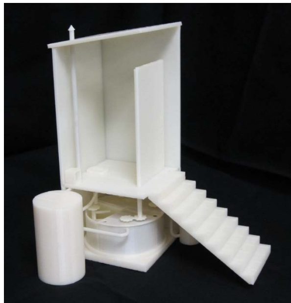
Figure 6. This composting toilet design was in response to a Gates Foundation Challenge. This design shows a perspective to highlight the novel modifications to current composting toilet designs. The external tank (bottom left) is part of the urine separation system. The composting carousel (bottom) is designed to collect the solids in the system and operate as a sequencing batch reactor (SBR). Unique to this design is that the SBR is mixed every time the door is open and shut.
