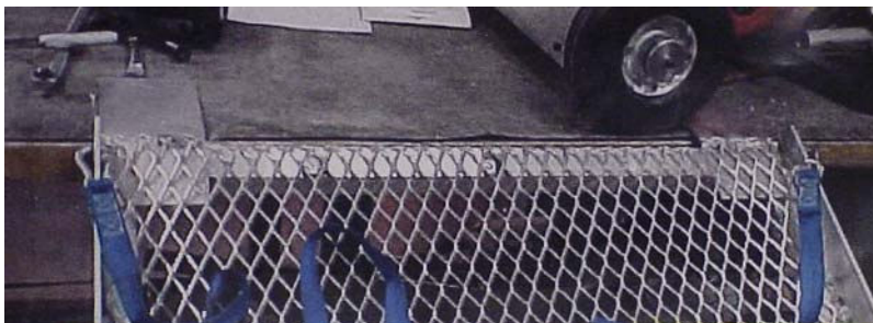
Figure 3. The Ramp with the “Paws” of the Pads Lying Flat on the Truck Bed. The Nylon Straps are to be Fastened in the Forward Stake Pockets or Side Rails in the Truck
