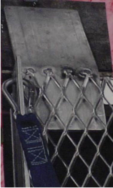
Figure 4. A Detailed View of the “Paws” or Pads that Help Connect the Upper End of the Ramp to the Truck Bed.
