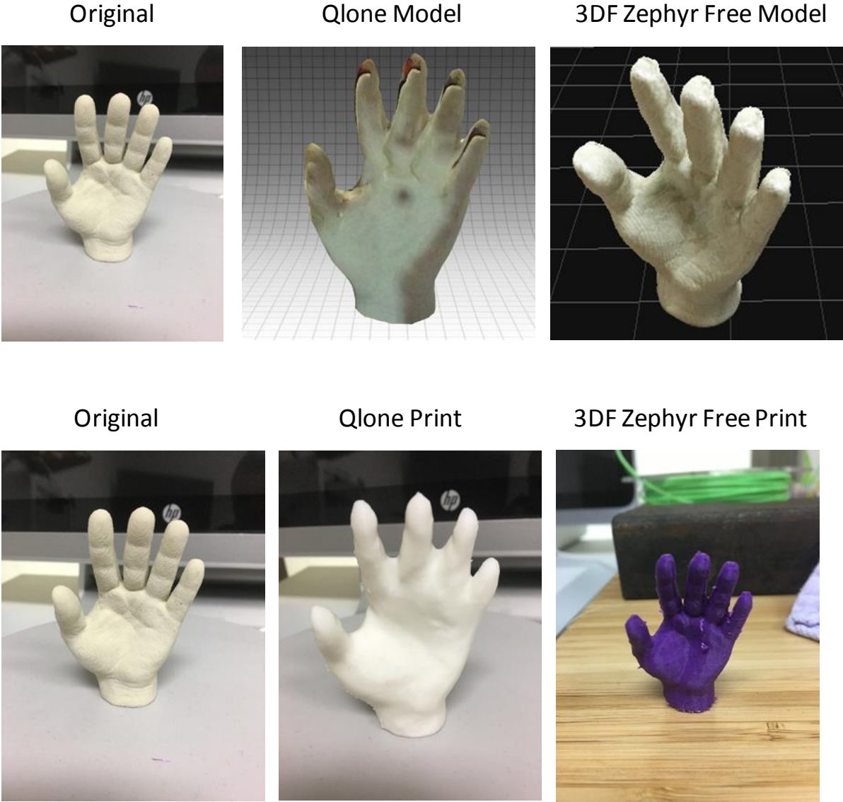
Figure 1: Qlone and 3DF Zephyr Free Software Tool Views of Left Hand (at the top) 3D Printed Views of Both Left Hands (at the bottom)
