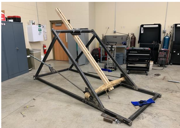
Figure 2. Completed torsion engine design (Version 1).
