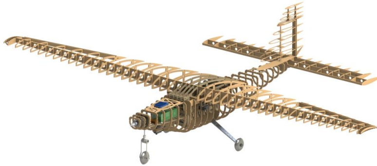
Figure a1: The airframe of the 2015 aircraft for the SAE Aero Design Competition 8
