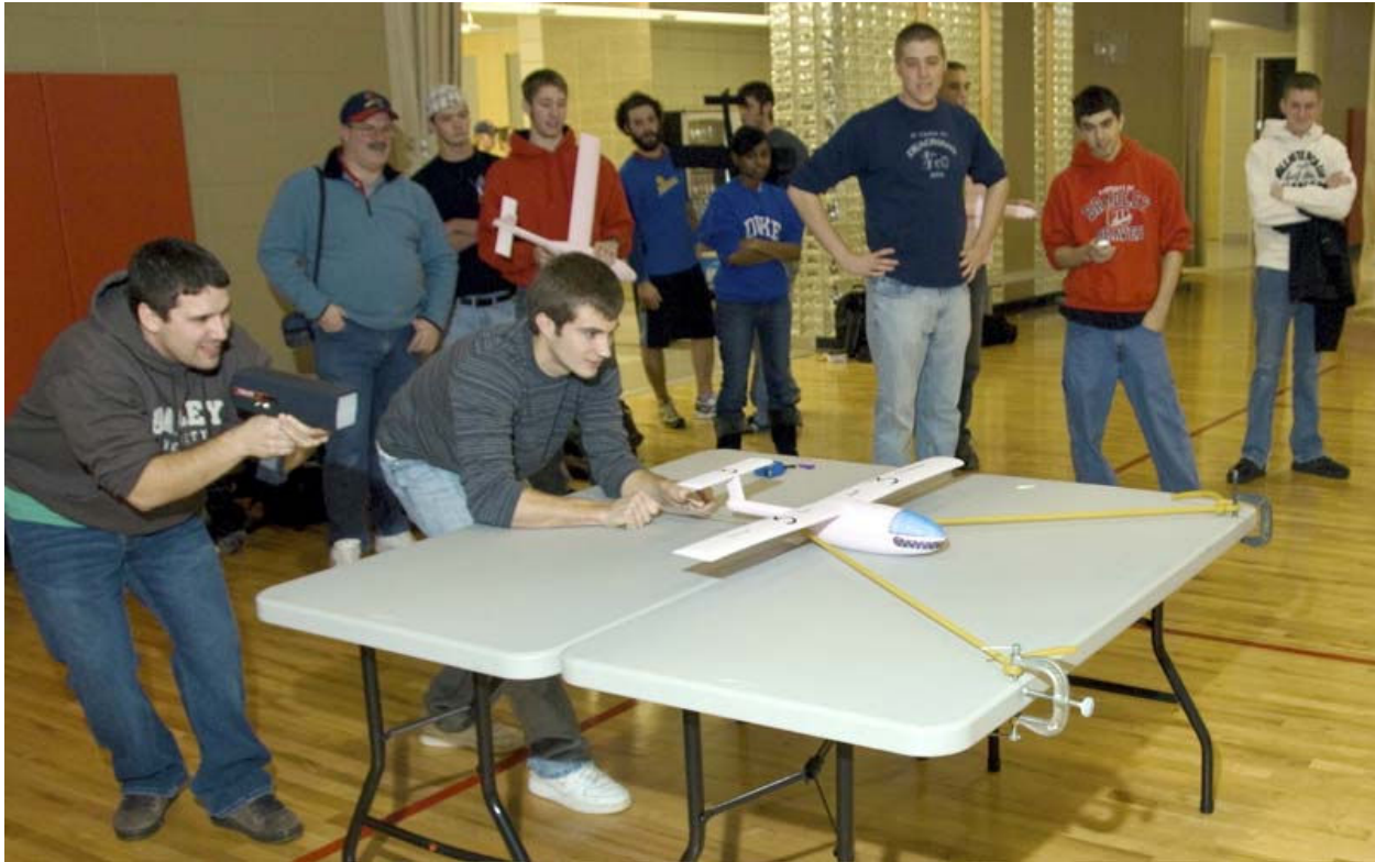
Figure 11: Final Launching. Initial launch speed was measured with a radar gun to confirm the initial launch velocity used in MATLAB simulations, which was found by measuring the spring constant of the elastic band.
