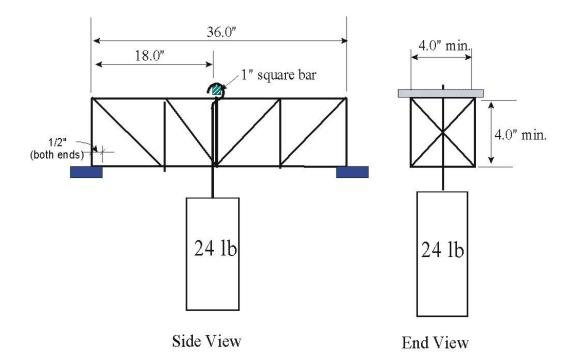
The object of this competition is to design and build a structure which is capable of supporting a load of 24 lb in the center of a 35" clear span, with 1/2" overlap at each support.
