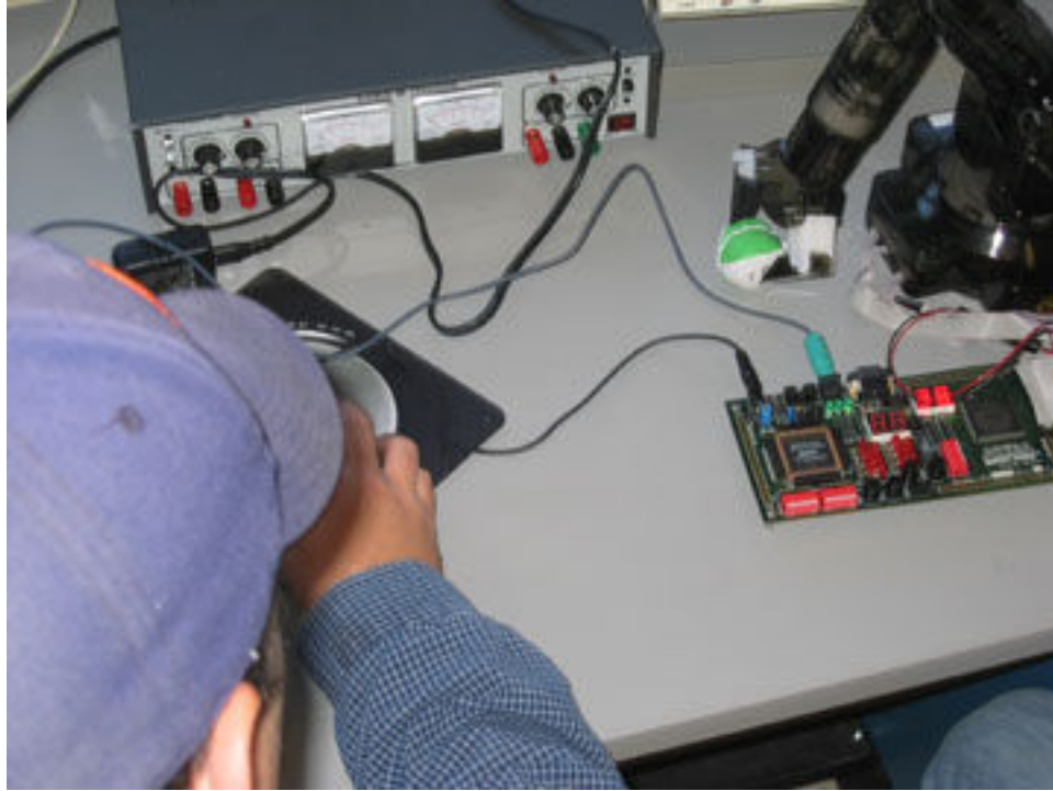
Fig. 3. Student using mouse to operate modified robot arm that holds ball. Altera UP-2 board(right center) is also shown.
