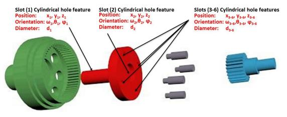
Figure 4: Features and feature slots of planet carrier
