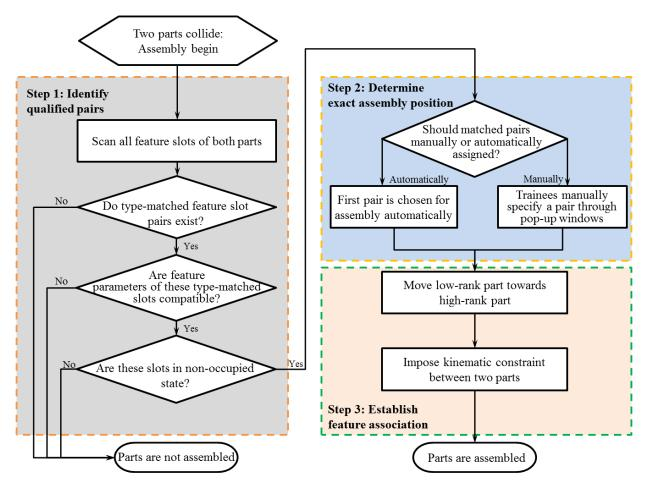
Figure 6 Flowchart of establishing a feature association after a trainee lets two mechanical parts collide
