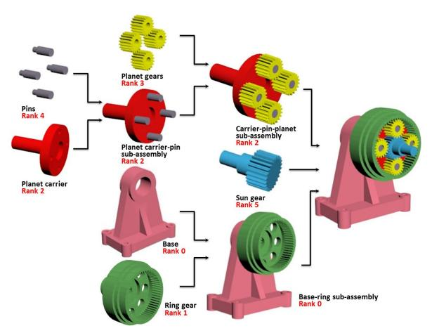
Figure 5: Hierarchy of gear train assembly
