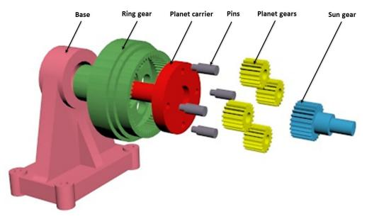
Figure 2: Exploded view of planetary gear train assembly
