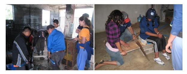
Figure 3a & 3b: Fabrication. The picture on the left was taken at the welders who assisted in attaching the frame to the bicycle tire rims. On the right, the students used resources from the community to construct the seat.
