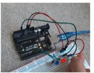
l put my fingers around the thermistor to increase the temperature, which caused the red LED to turn on and the blue one to turn off.
