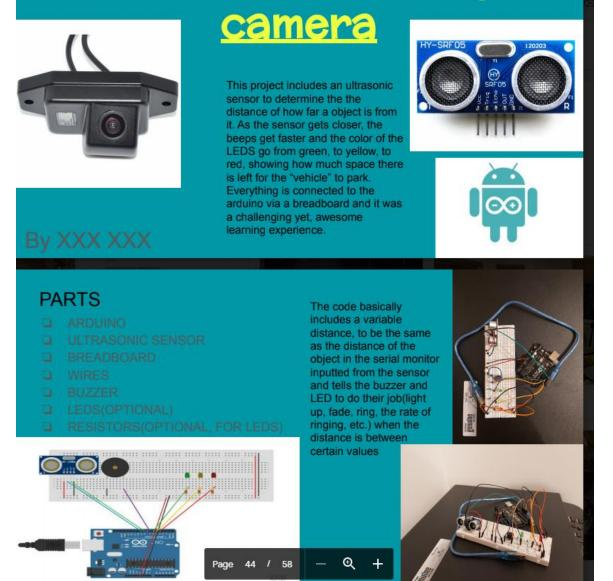
Figure 2: Use of both Tinkercad and a real Arduino for an ultrasonic sensor project.
