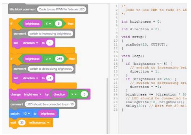
*Figure 3: Tinkercad has both text coding (right) and code blocks (left). When using code blocks, Tinkercad also creates the text verson.*
