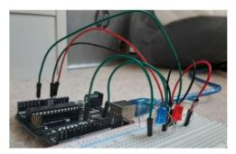
For this project, I used a thermistor, 2 LEDs, 3 resistors, 7 wires, and of course a breadboard as well as the Arduino UNO. My goal was to make the blue LED light turn on when the temperature was low and make the red LED turn on when the temperature was high.
