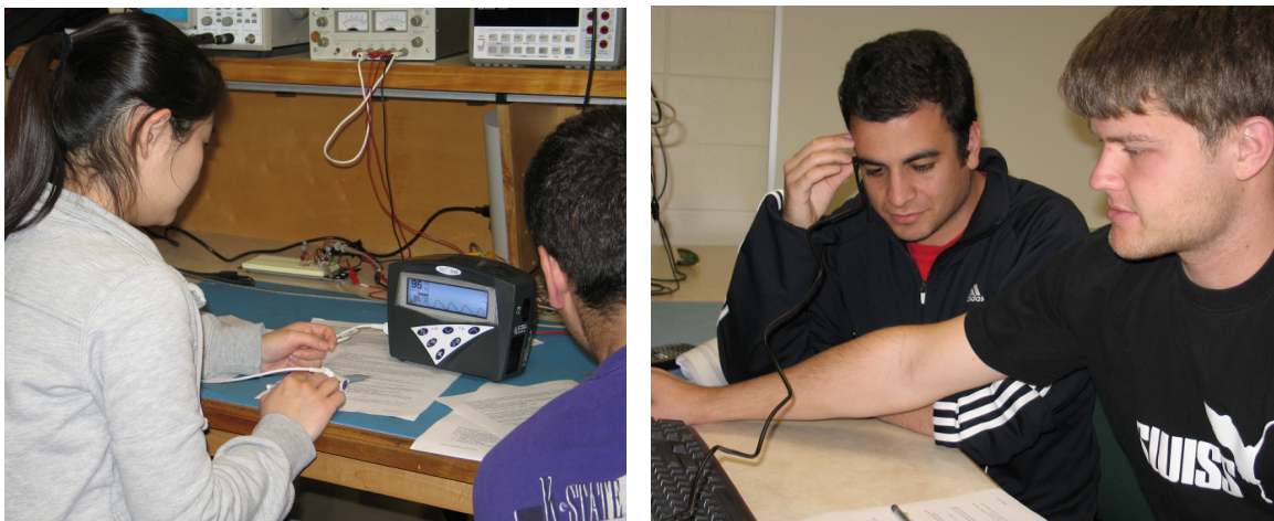
Figure 6. Blood oxygen saturation determination using the BCI ® 3180 pulse oximeter (left) and photo-plethysmogram measurement on the temple to assess respiration rate (right).
