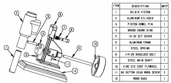
Figure 3: Air Motor Exploded Assembly Drawing
