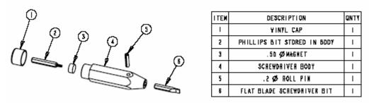
Figure 2: Screwdriver Assembly
