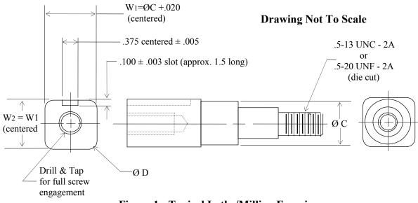
Figure 1: Typical Lathe/Milling Exercise
