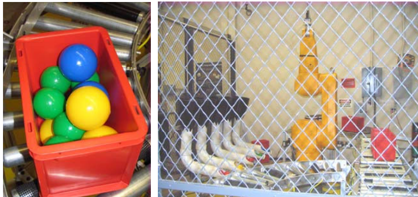
Figure 10: Shipping container with ball order fulfilled and complete sorting system
