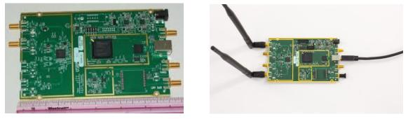
Figure 4. USRP B200 (left) and B210 (right).
