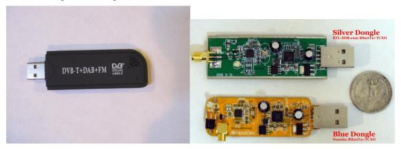
Figure 1. RTL-SDR USB Dongle. [www.radioforeveryone.com, Dec 22, 2016.]
