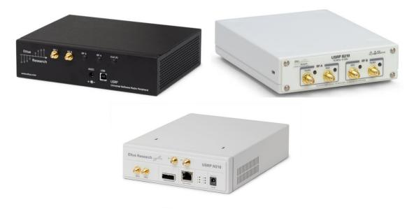
Figure 5. Metallic enclosures for the USRP1 (left), B200/210 (right) and USRP N210 (bottom).
