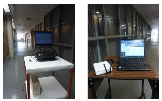
Figure 8. Indoor transmitter-receiver set-up for the mobile platform
