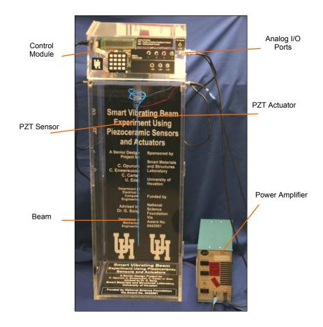
Figure 1: Smart Flexible Beam Experiment
