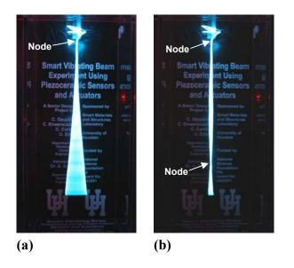
Figure 4: (a) First and (b) Second Mode Operation of Smart Flexible Beam
