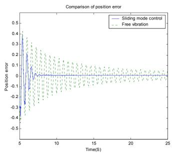
Figure 6: Comparison of Beam in Free Vibration and Beam with Sliding Mode Control
