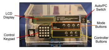
Figure 3: Smart Beam Control Module
