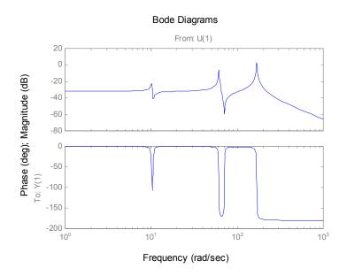
Figure 5: Bode Plot of Smart Flexible Beam System
