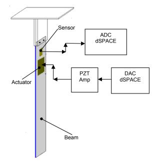
Figure 2: Schematic Operation of Flexible Beam
