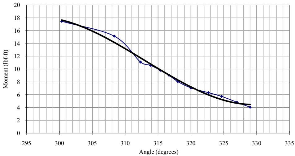
Figure 10 Moment of a torsion bundle vs. Angle for the second configuration
