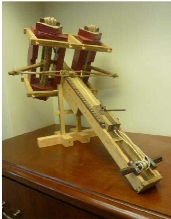
Figure 1 The form of the ballista that is described by Heron and Philon.
