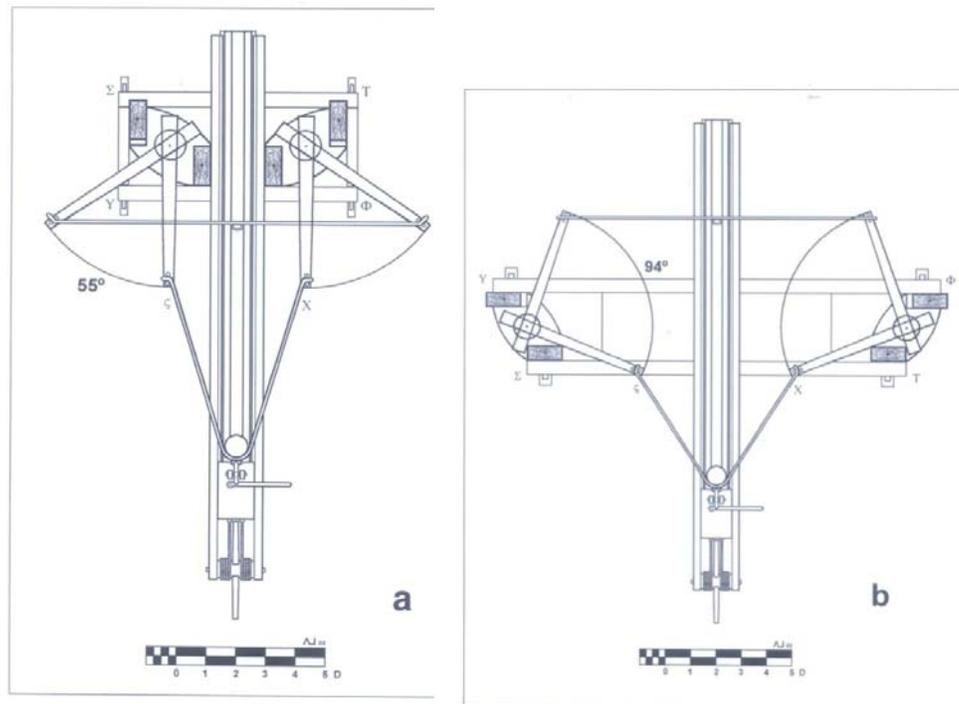
Figure 4 The two principal ballista configurations: the out swinging (a) and the in swinging forms (b).
