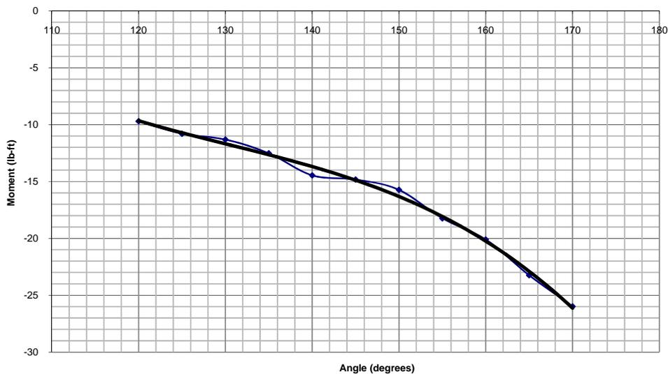
Figure 11 Moment of the torsion bundle vs. Angle for the third configuration
