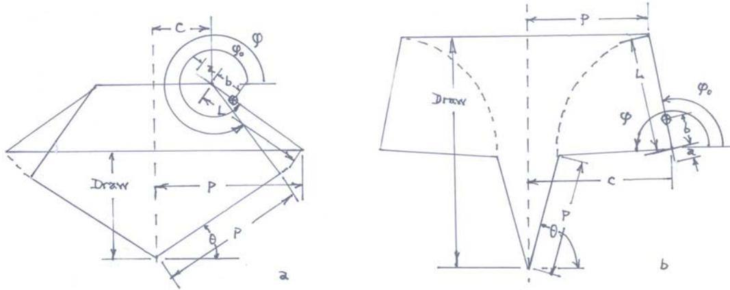
Figure 8 Geometry used in the analytic analysis (a) for the first and second configuration and (b) used for third configuration.
