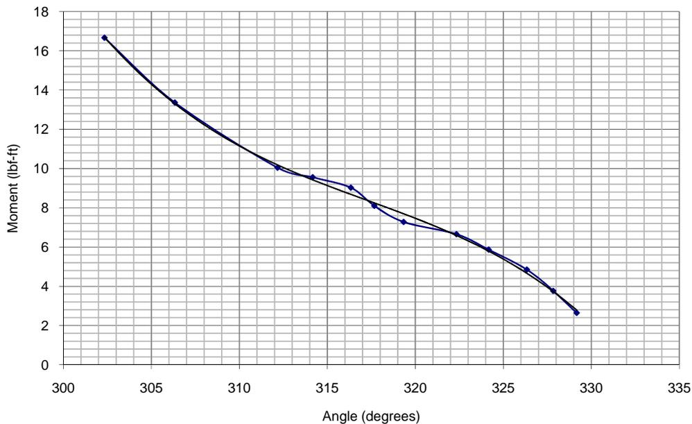
Figure. 9 Moment of a torsion bundle vs. Angle of twist for the first configuration
