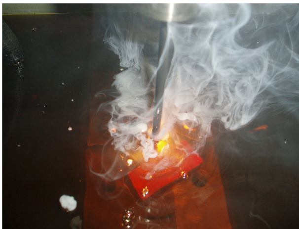
Figure 2. Carbon nanotube production using an electric discharge machine
