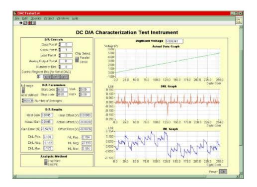
Figure 2. Linearity testing of a digital-to-analog converter.
