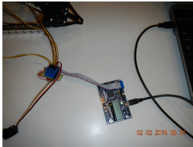
Figure 17: The USB connection between the PC and the Atmel board.
