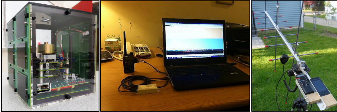
Figure 6 - EyaSat Classroom Satellite Kit, Packet Radio Communication, Handheld Radio and Antenna (Portable Radio Communication)
