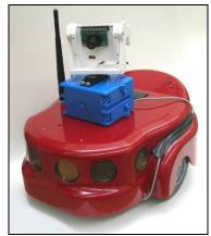
Amigobot. The cameral was used for obstacle avoidance and path following.
