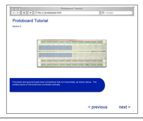
Figure 3: Screen shot of an on-line interactive demo for the use of a virtual protoboard.
