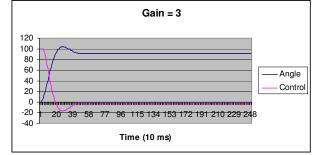
Figure 5: LEGO NXT motor control experiment. Students can enter a gain directly in the NXT processor interface and run the motor position controller with different levels of gains. They can try to turn the motor away from its set point and find that the higher the gain, the harder it is to turn the motor from its set point
