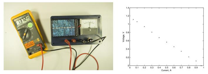
Figure 7: Solar panel experiment to measure I-V curves, on left, with resulting I-V curve, on right.
