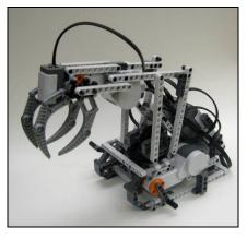
Figure 8: Term project completed with the Figure 9: Term project completed with the LEGO NXT, this robotic arm was interfaced with another LEGO NXT mobile robot to perform coordinated tasks using wireless communications.
