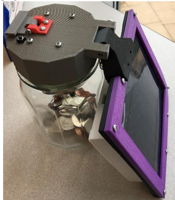
Figure 6 – Photograph of the solar-powered piggy bank accountant. This project had more mechanical design than many as the different size coin are diverted to different sensors for counting when they are inserted.
