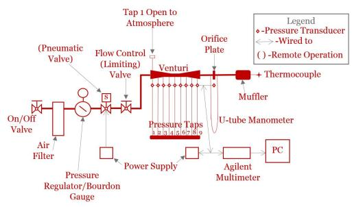
Figure 1: Venturi Flow Experiment Schematic
