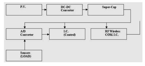
Figure 3 Harvester block diagram
