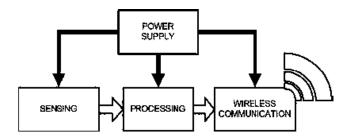
Figure 1. Block diagram of a sensor node
