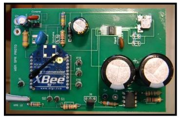
Figure 4 Energy harvesting circuit
