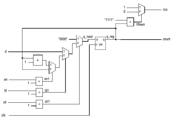
Figure 9. Conceptual diagram of a 74163-like counter
