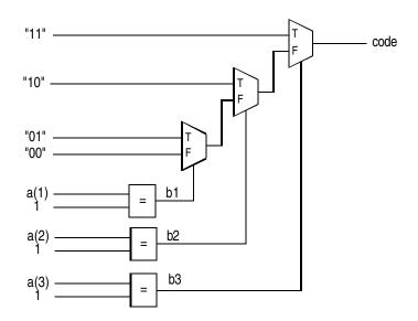
Figure 5. Module-level implementation of 4-to-2 priority encoder
