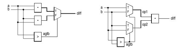
Figure 6. Block diagrams of two difference circuits
