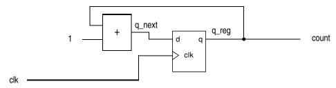
Figure 8. Conceptual diagram of a free-running binary counter
