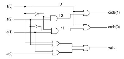
Figure 4. Gate-level implementation of 4-to-2 priority encoder
