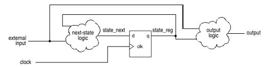
Figure 7. Conceptual diagram of a synchronous sequential circuit
