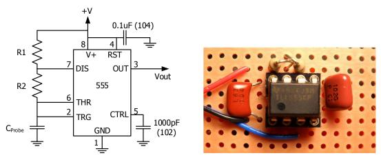
Figure 2. 555 Timer Oscillator Circuit Schematic and Suggested Circuit Board Layout
