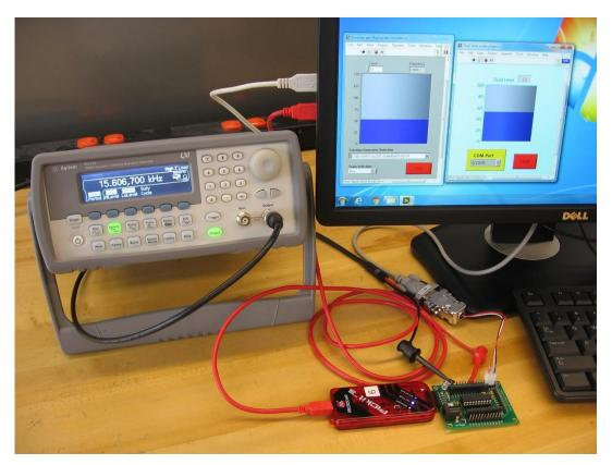
Figure 9. Hardware In the Loop testing setup
