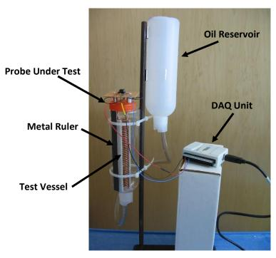
Figure 4. Probe test and calibration setup
