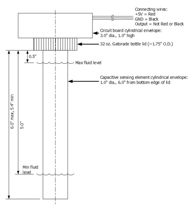
• External connecting wires must be 12" +/- 1" long, stranded (not solid) of #22 - #26 AWG. Colors as shown on diagram.
