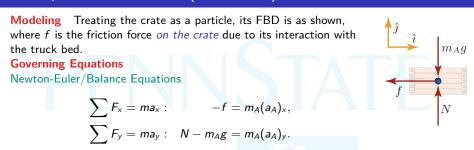
Material Models Since we want the *minimum* coefficient of static friction between the crate and truck required for no sliding, that means that slip must be impending and so
