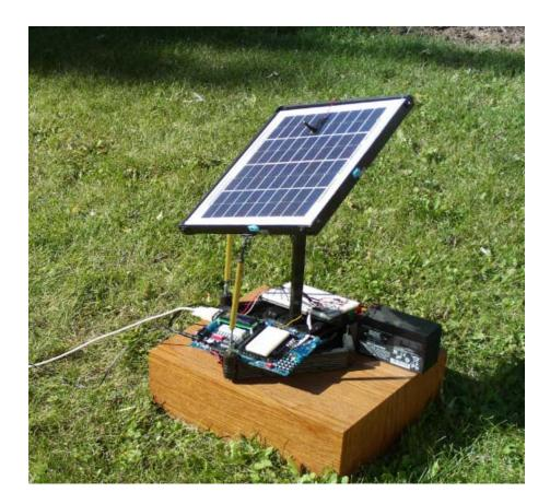
Figure 2. Project prototype of Portable Self-powered Solar Insolation Measurement System
