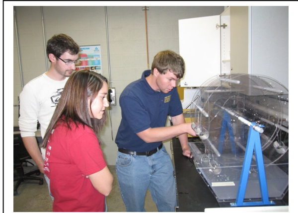
Figure 1. Laboratory device for soaking and drying corrosion test specimens.
