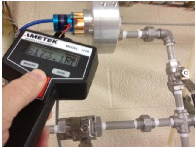
Figure 7. RPM measurement on our Tesla turbine.
