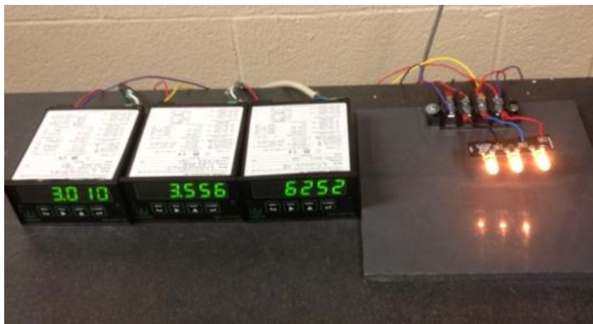
Figure 8. Electrical signal measurements (A, V, RPM) and light output from our turbine.
