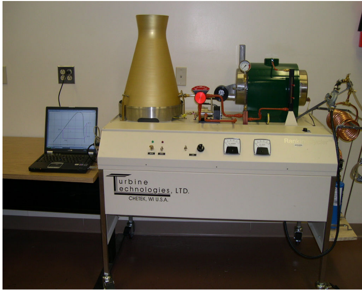
Fig 5. Propane fueled steam engine cycle
