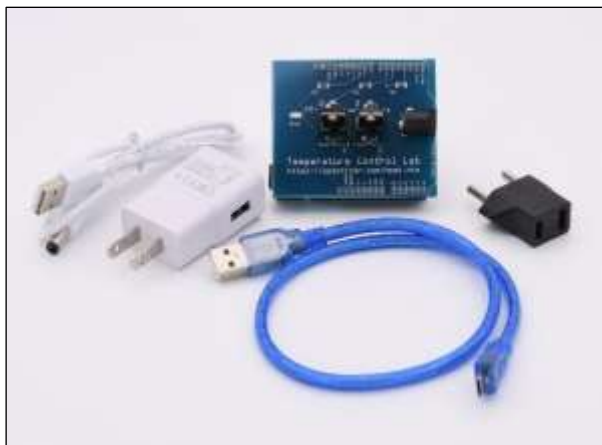
Figure 2: Temperature Control Lab (TCLAB) Kit (Arduino based)
