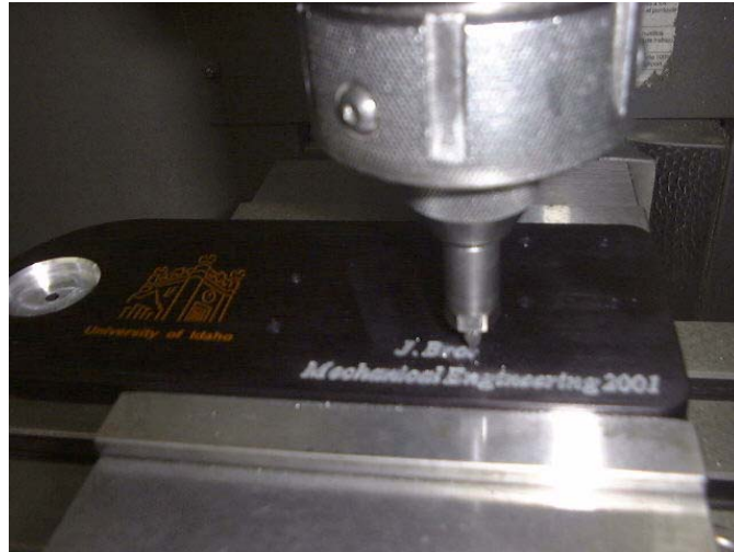
Figure 5. CNC engraving a student's engine base plate.
