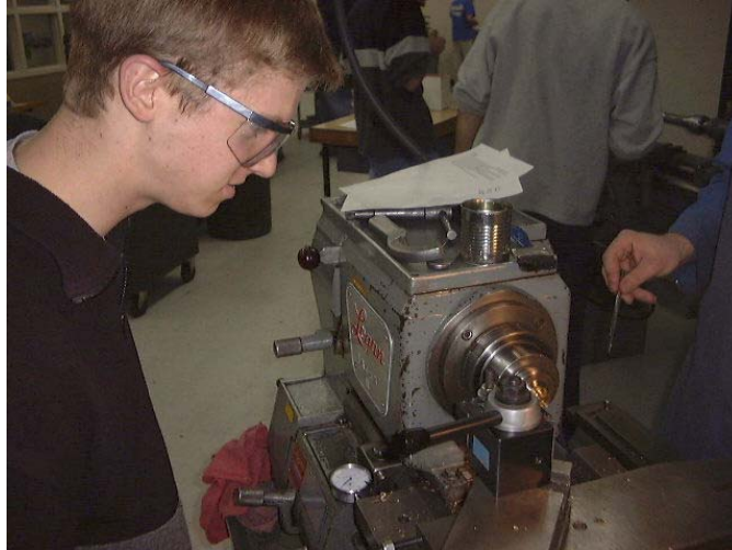
Figure 4. Student cutting O-ring groove in alcohol burner cap on a manual lathe.
