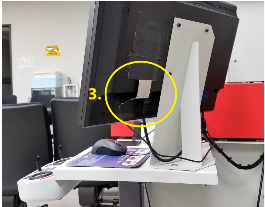
Figure 3. Close-up of (3) from Figure 2. The audio notification hookup is attached near the built-in speaker on the monitor.
