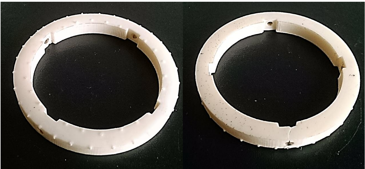
Figure 1. Gimbal assembly produced on the VFlash FTI system showing residual nubs from the support structure on surfaces facing the build plate (left) and the smooth surfaces which were oriented away from the build platform.
