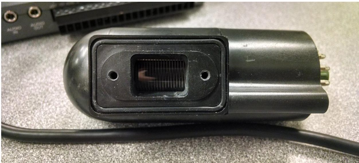
Figure 2. Photomultiplier tube showing the aperture without bandpass filter or filter cover.
