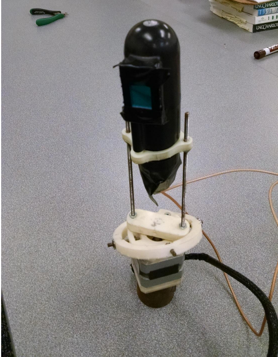
Figure 6. Photomultiplier Tube (PMT) mounted on the gimbal and stepper motor
