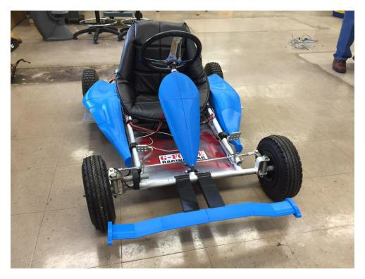
Figure 7: Electric go-kart with 3D printed body parts
