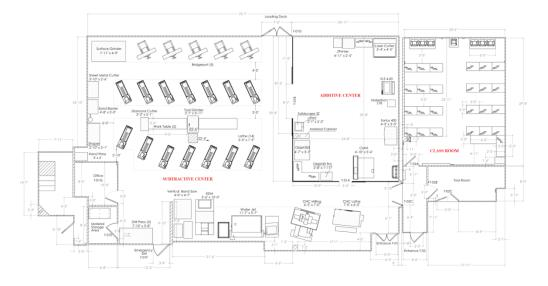
Figure 4: Floor plan of the Advanced Manufacturing Laboratory
