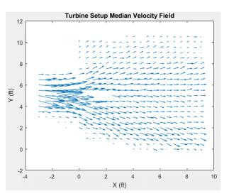
Figure 9: Anemometer and fan are Figure 10: Velocity field showing the flow disturbance caused by the wind turbine.
