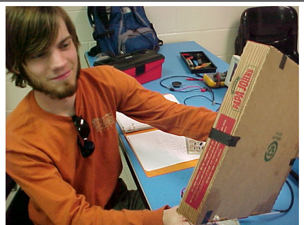
Figure 5: Square-loop antenna realized on a pizza box.
