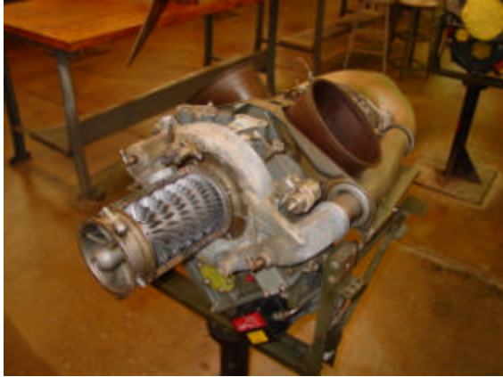
Figure 8 PT6-A cutaway engine
