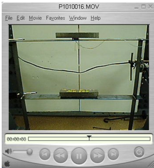
Figure 20 Frame with Additional Masses on Beams
