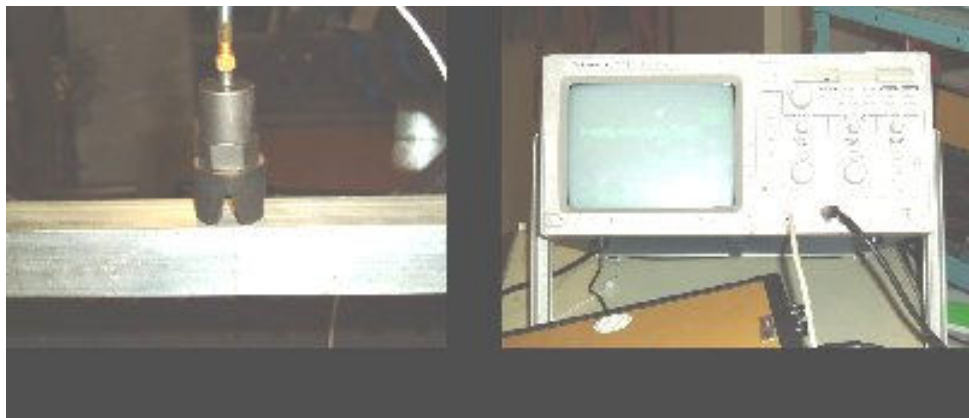
Figure 5 Aluminum beam, accelerometer and oscilloscope
