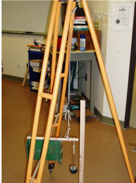
Figure 3: Setup for the Rotational Single Degree-of-Freedom System
