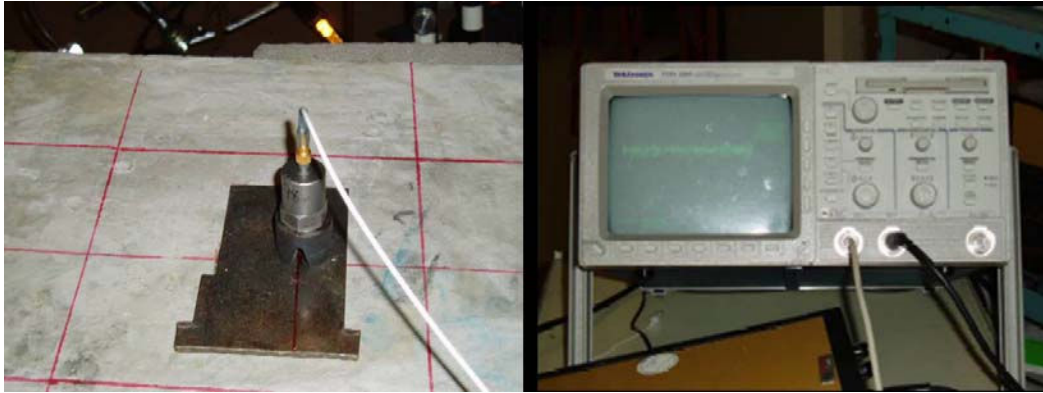
Figure 11. Accelerometer at L/4 and Oscilloscope on the Reinforced Concrete T-Beam
