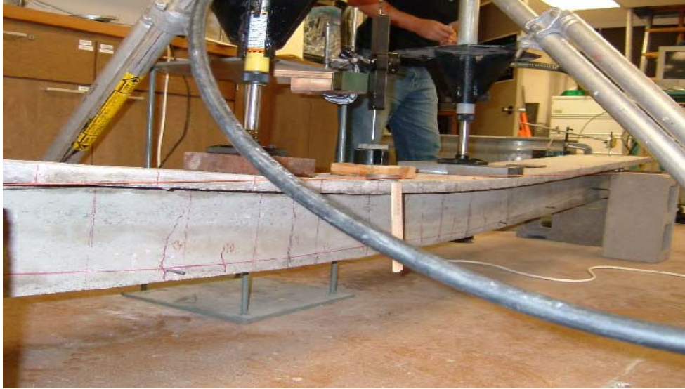
Figure 14. Setup of the static test and cracks of the Post-Tensioned Concrete T-beam
