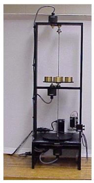
An unrestrained torsional mechanical system
