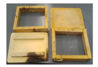
Figure 3. The Flask (cope and drag, bottom board, and pattern board)
