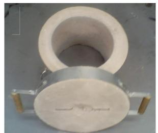
Figure 4. Crucible components for Melting Aluminum
