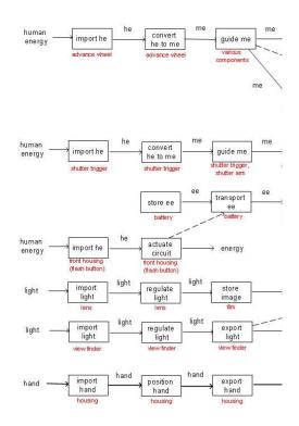
Figure 7. Function structure model of a Kodak disposable camera.
