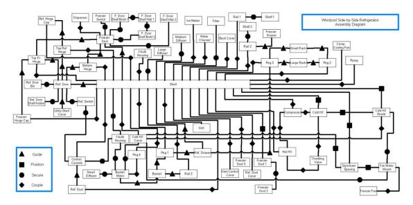
Figure 6. Assembly model of a side-by-side Whirlpool refrigerator
