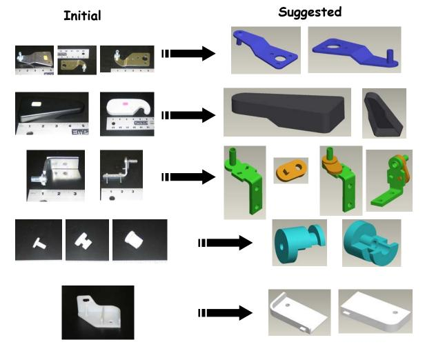
Figure 5. Redesigned components from the Whirlpool refrigerators using ProEngineer.
