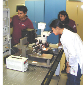
Figure 2. (Left) Student-team-designed Silicon Germanium 5-6 GHz Voltage Controlled Oscillator. The fabricated circuit is being measured using RF on-wafer probes. (Right) Student team conducting on-wafer measurements on their fabricated circuit.
