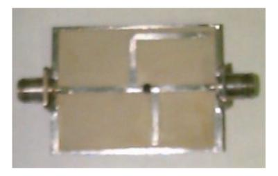
Fig. 6. Picture of the final Cellular Band Power Amplifier.
