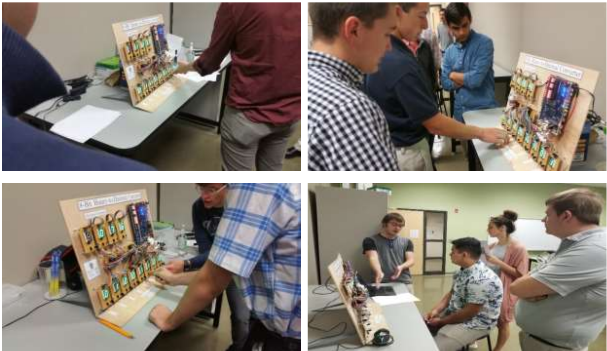
Figure 6: Students using the B-To-D Emulator to practice converting decimal integers into binary equivalent representation.
