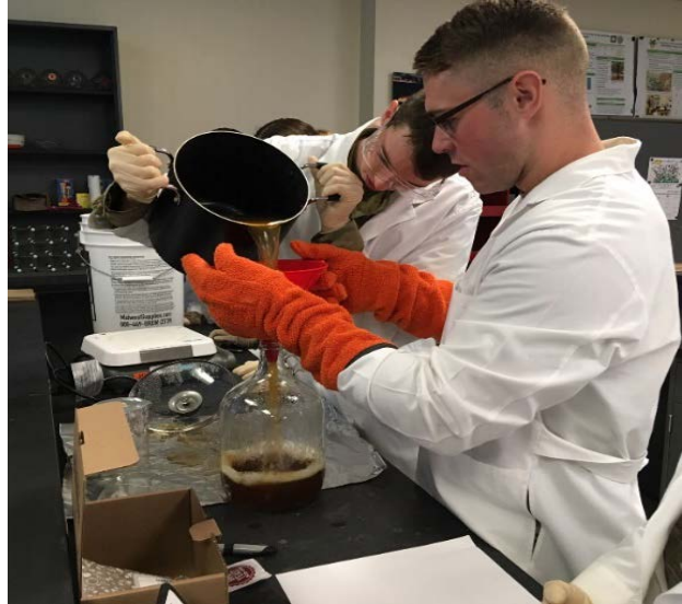
Figure 5. EV396 students engaged in hands-on learning while aseptically transferring the prepared wort mixture into a glass fermenter where the 14-day fermentation process will ensue.
