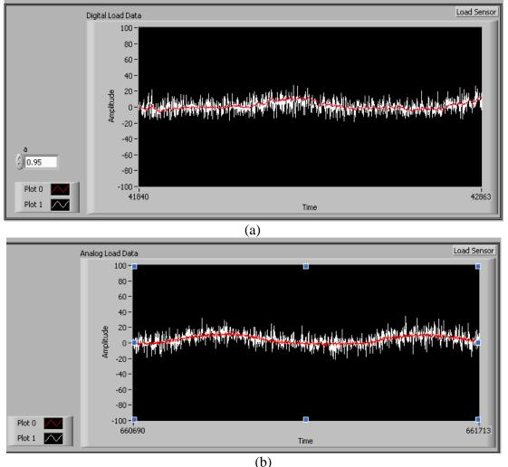
Fig. 2. Raw vs. filtered signals (digital (a) and analog (b) filters)
