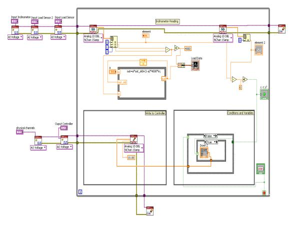
Fig. 3. LabVIEW front panel for pump jack control system
