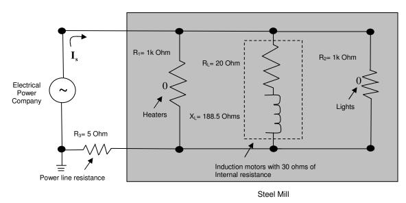
Figure 2: Power Factor Correction Practical Exercise Circuit
