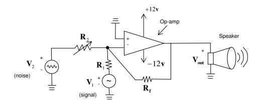
Figure 4: Signal-to-Noise Ratio Practical Exercise Circuit
